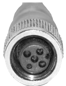
CLOSE-UP Station Communication Cable Connector
