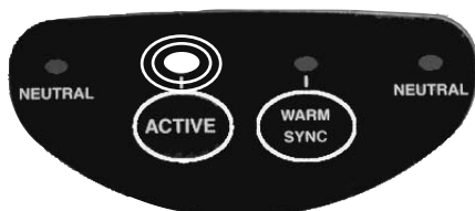
ACTIVE light is flashing at station that is INACTIVE
