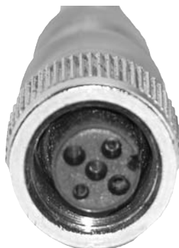
CLOSE-UP Station Communication Cable Connector
