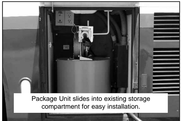
Package Unit slides into existing storage compartment for easy installation.
