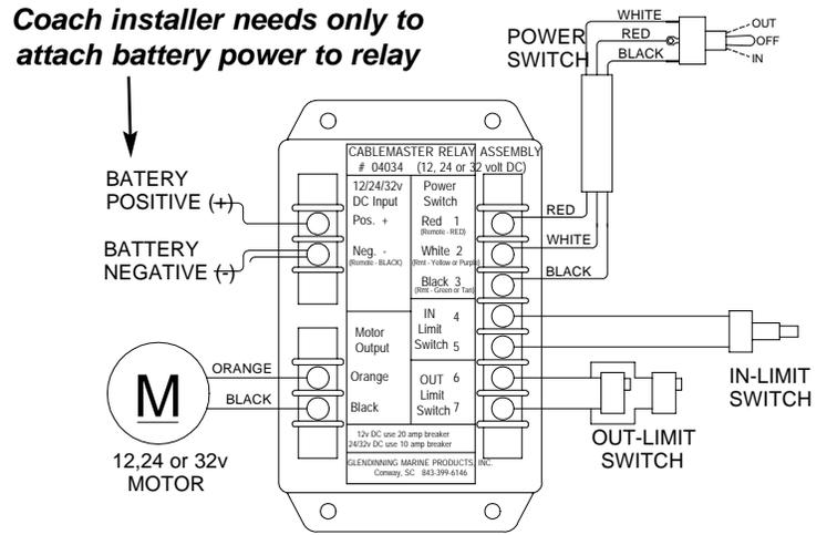
SECOND, attach battery power leads to the red (positive) and black (negative) wires on the RVCM-LC power unit.
