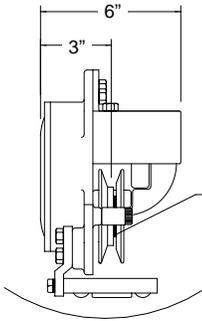
NOTE: SPACERS PROVIDED FOR VARIABLE CABLE DIAMETER ADJUSTMENT
