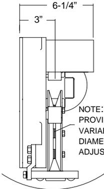
NOTE: SPACERS PROVIDED FOR VARIABLE CABLE DIAMETER ADJUSTMENT
