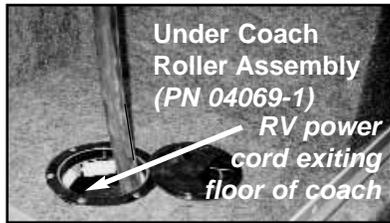
The second step is determining where the cable plug will exit the interior of the coach. In many coaches, the cable exits through an access hole on the bottom of the cable storage area or electrical hookup bay (see photo at left). In other cases, the power cable may exit the side of the coach through a new or existing access door (similar to a fuel door, see above). In either case, a route must be identified that the cable will take from where it is stored to the outside of the coach.
