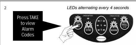
Pressing the TAKE button will allow you to cycle through the 16 most recent alarm codes. Record the sequence of blinking LEDs on page 5. Determine the alarm code by using the chart on pages 6-7 and fill in the appropriate space on the chart.
