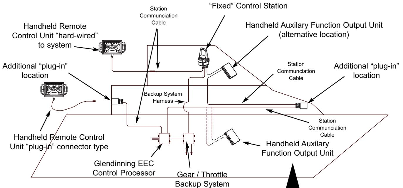
The Handheld Auxiliary Function Output Unit communicates between the handheld control buttons and the control circuits for bow or stern thruster, engine start or shutdown, and / or rudder control and can be located in the engine compartment near the control processor or near any control station where interfacing with other control functions is easier.
