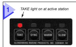
**ACTIVE STATION—**During normal operation only Active Station will be in command. TAKE light stays on (fully illuminated) indicating that station is active and in command.
