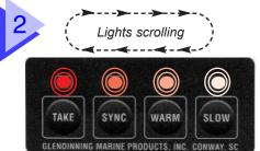
**TURN ON EEC** power switch. **DIAGNOSTIC TEST** will be performed by the EEC System (indicated by scrolling lights across panel). Do not move handles while lights are scrolling).
