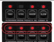
IF TAKE, WARM AND SLOW LIGHTS ARE ON—control handles are not in neutral. Leave control system power switch on and move one control handle at a time to verify that the handles are in neutral position. When both handles are in neutral, indication lights will begin to scroll (as in Step #2 above).
