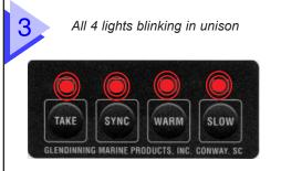
**ALARM MODE**—During normal operation, the EEC system continuously monitors parameters and will alert operator of alarm conditions (indicated by all 4 lights blinking in unison.)
