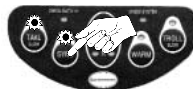
SYNC LIGHT WILL GO OUT WHEN SYNC MODE IS TURNED OFF—EEC SYSTEM IS NOW IN NORMAL CRUISE MODE.
