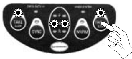
TROLL LIGHT WILL GO OUT WHEN TROLL MODE IS TURNED OFF—EEC SYSTEM IS NOW IN NORMAL CRUISE MODE.
