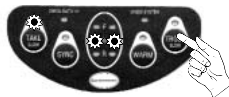
TROLL LIGHT WILL BE ILLUMINATED WHEN EEC SYSTEM IS IN TROLL MODE
