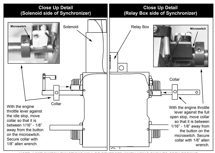
NOTE: LIMIT SWITCH FUNCTIONS WILL BE REVERSED WHEN USING PUSH-TO-OPEN FORMAT
