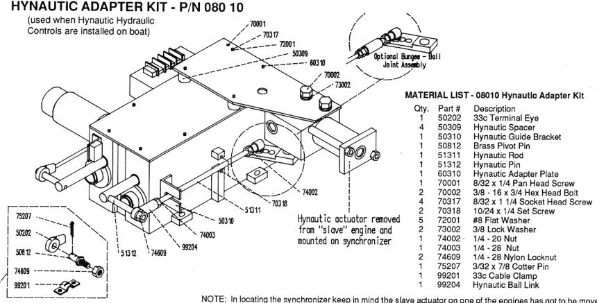
Installed at slave engine governor
