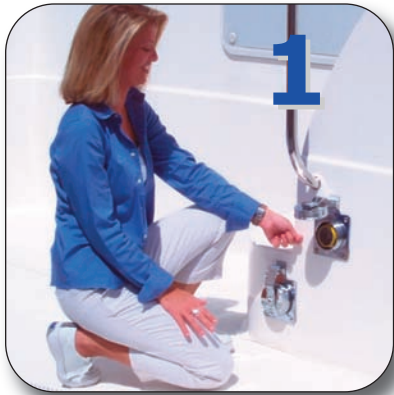
Open Hawse Pipe cap and lock in upright position
