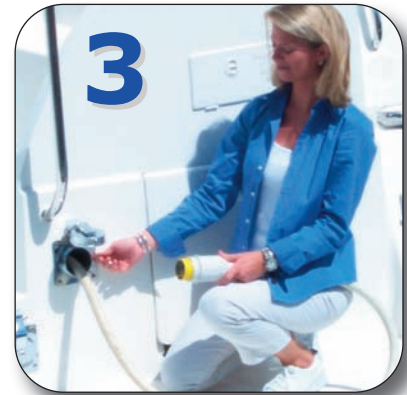
Turn off power switch when desired cable length has extended.
