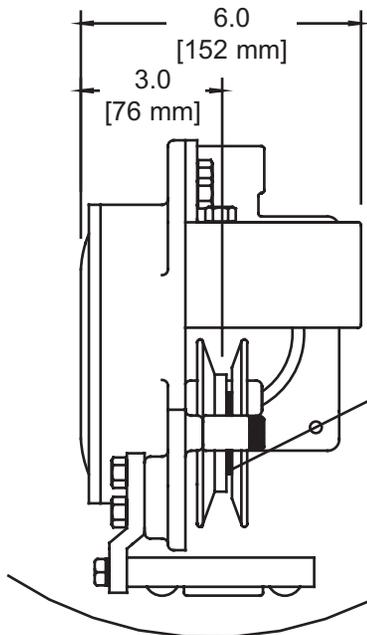
NOTE: Spacers provided for variable cable diameter adjustment
