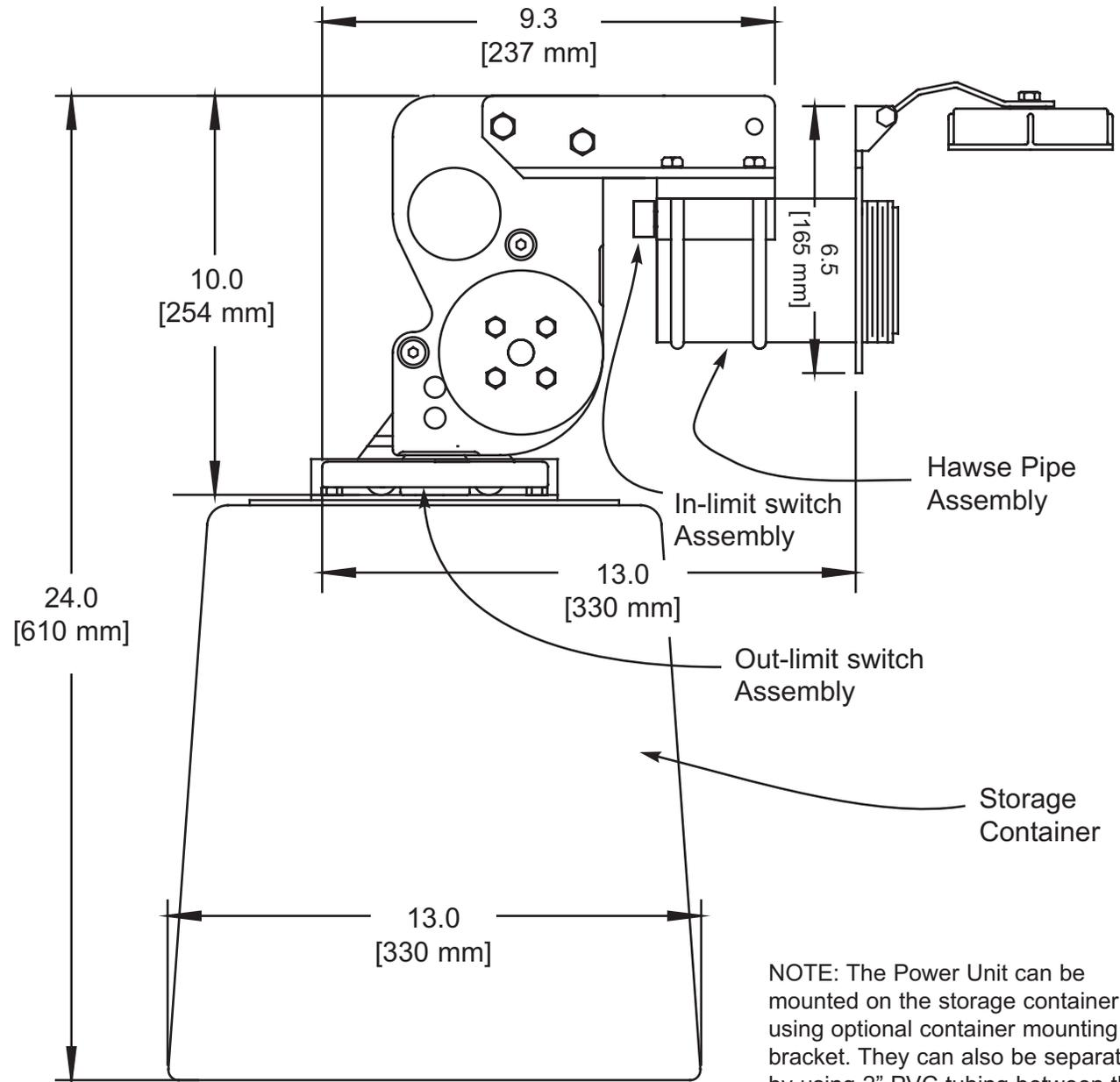
NOTE: The Power Unit can be mounted on the storage container using optional container mounting bracket. They can also be separated by using 2" PVC tubing between the Container and Power Unit.
