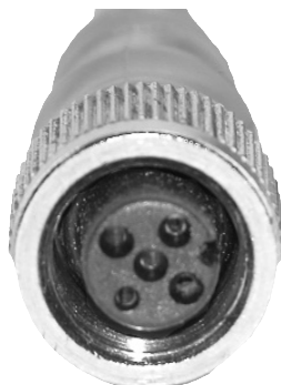
CLOSE-UP Station Communication Cable Connector
