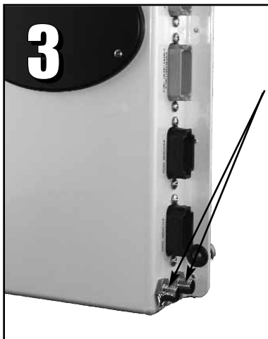
Photo 3 Control Processor station connection points.
