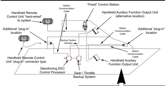
The Handheld Auxilary Function Output Unit communicates between the handheld control buttons and the control circuits for bow or stern thruster, engine start or shutdown, and / or rudder control and can be located in the engine compartment near the control processor or near any control station where interfacing with other control functions is easier.
